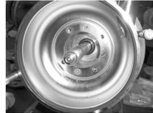
Abb. 39 Stationary ring of mechanical seal
