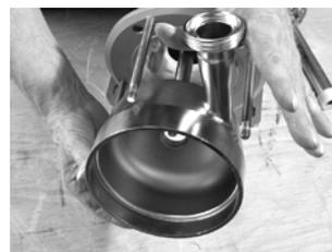
**Abb. 36** Discharge casing / bearing housing
