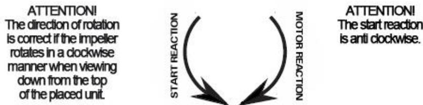
With bigger pumps the check may be done by watching the rotation of the impeller through the discharge or suction inlet. Switch the pump on and off and check the direction of rotation when the impeller rotates slowly.
