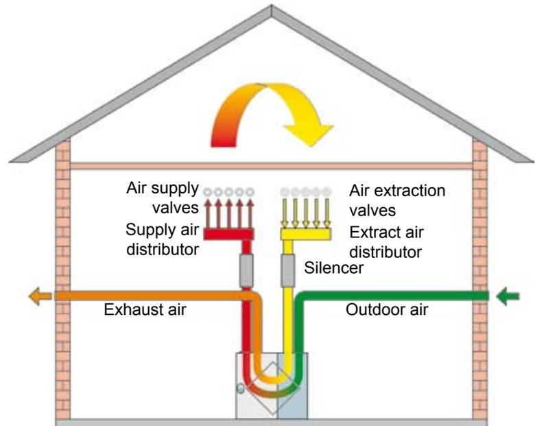
For setting up the outdoor air and exhaust air ducts from and to the CWL Comfort home ventilation unit.
