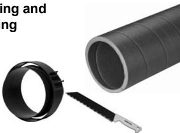
The insulated pipes can be shortened as required using the fitting knife and can be joined using clamping rings. This makes it possible to carry out laying with virtually no wastage of material.
